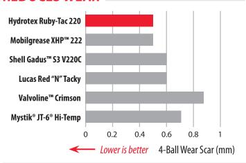
The 4-Ball Wear Scar Test measures how well a grease lubricates and protects components against wear. Ruby-Tac 220 provides best-in-class wear protection.
