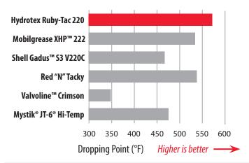
The dropping point is the temperature at which a grease transitions from semi-solid to liquid and it is one indication of a grease's heat resistance. Ruby-Tac 220 exceeds competitor dropping points.
