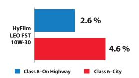
Fleet Testing conducted according to the EPA Federal Test Procedure (FTP) demonstrates significant fuel economy improvement over all driving scenarios when switching to HyFilm FA-4.
