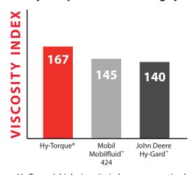
Hy-Torque's high viscosity index ensures optimal lubrication over a wide temperature range for consistent all-season performance.
