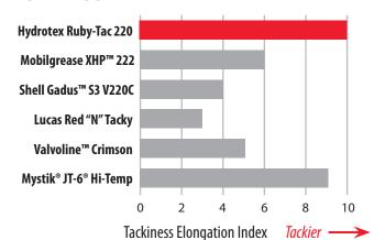
The Hydrotex tackiness elongation index is a measure of the adhesivecohesive "stringiness" of a grease and indicates its ability to effectively travel though moving systems and create a protective coating.
