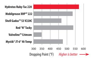
The dropping point is the temperature at which a grease transitions from semi-solid to liquid and it is one indication of a grease's heat resistance. Ruby-Tac 220 exceeds competitor dropping points.
