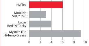
Elongation is a measure of the adhesive-cohesive "stringiness" of a grease and indicates its ability to effectively travel through moving systems and create a protective coating.
